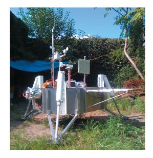
aluminum tubes and pairs of aluminum outriggers that join together at three foot pads. The foot pads are made of aluminum honeycomb material sandwiched between two outer layers of graphite impregnated epoxy. The leg system distributes the load from the foot pad to the lower corners of the body and to a point above the body at the top of the mounting post. This system allows the lander to remain stable under any surface conditions.
