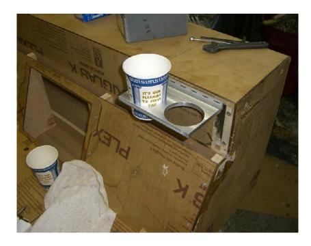
test weight on unit, then check for stress cracks or bending.
